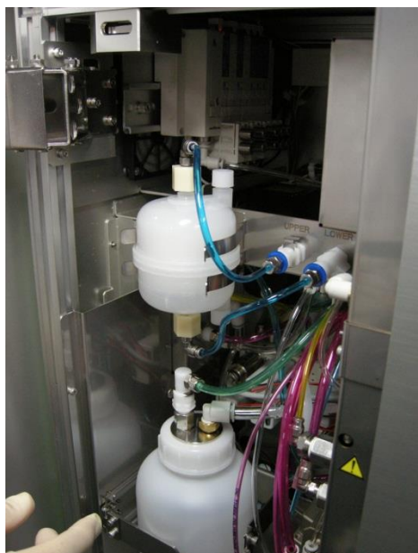
Sheath filter (inside fluidics maintenance door on left side of main unit)
