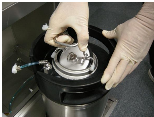
Sheath tank lid
